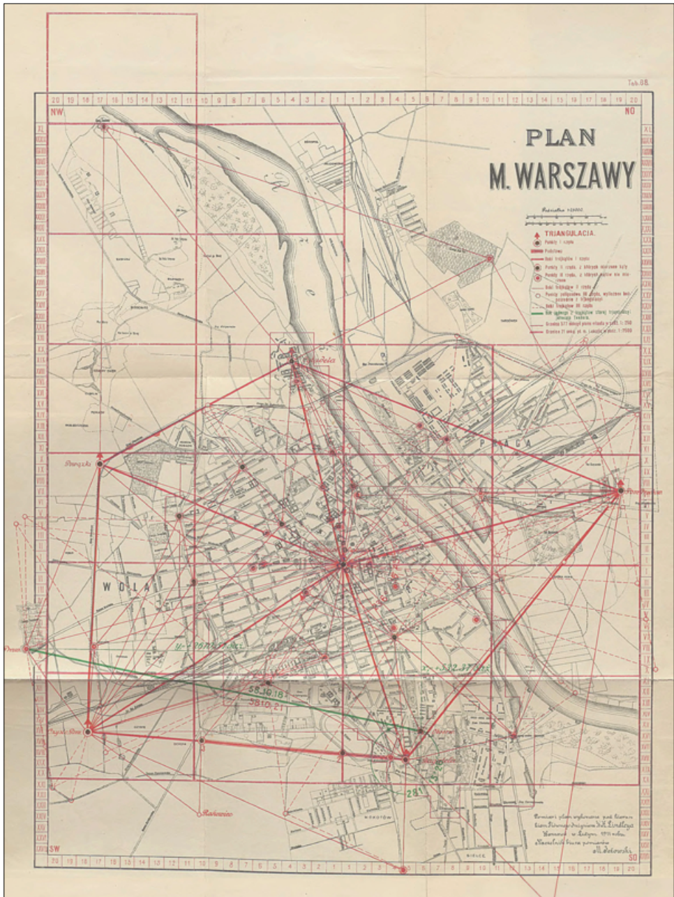
Fig. 1. Triangulation and polygonisation developed for the needs of measurement plans and maps. This sketch shows how the 1:2,500 map was divided into 21 sheets. Description in the lower right corner: "Measurement and plan made under the direction of Chief Engineer W. H. Lindley Warsaw in February 1911, Head of the Office of Measurements M. Jeżowski". Source: M. Jeżowski, "Rozdział XV", Tab. 68; public domain
